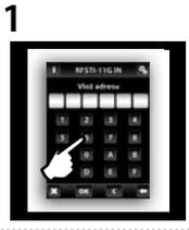
On the RF Touch, the address is requested of the required monitoring actuator RFTI-10B (RFTC-10/G), modified by an offset.
