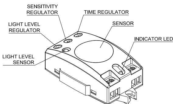
The ECOMAT MINI movement detector is capable of detecting the slightest movement because of its high-frequency technology. Its detection precision does not depend on the ambient temperature. It immediately detects any movement, even those of inert elements, such as doors or chairs.
