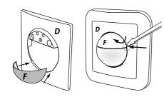
For outdoor installations additionally the IP54-accessory-fixing-set has to be mounted (Part nr. 92139).
